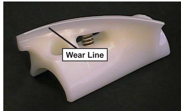
Figure 3-3 Auger Flight Wear
