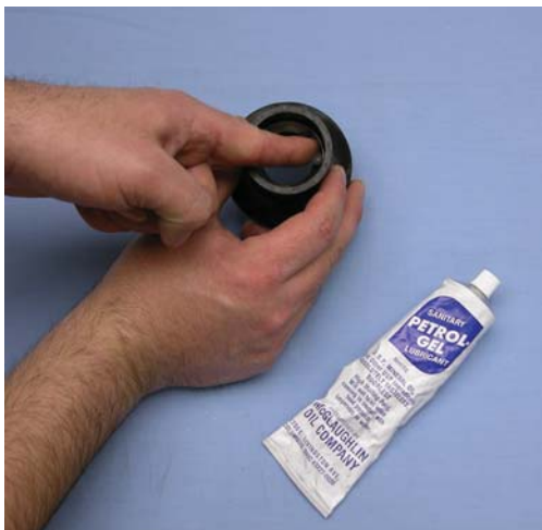
Figure 3-6 Lubricate Rear Seal
